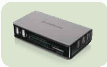
GUH286 5-Port USB 2.0 Hub and 56-in-1 Card Reader with Mini-B Charging Cable
